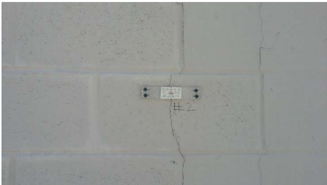
Photo 3: Crack gauge 2 position on a vertical crack on the north exterior wall.
