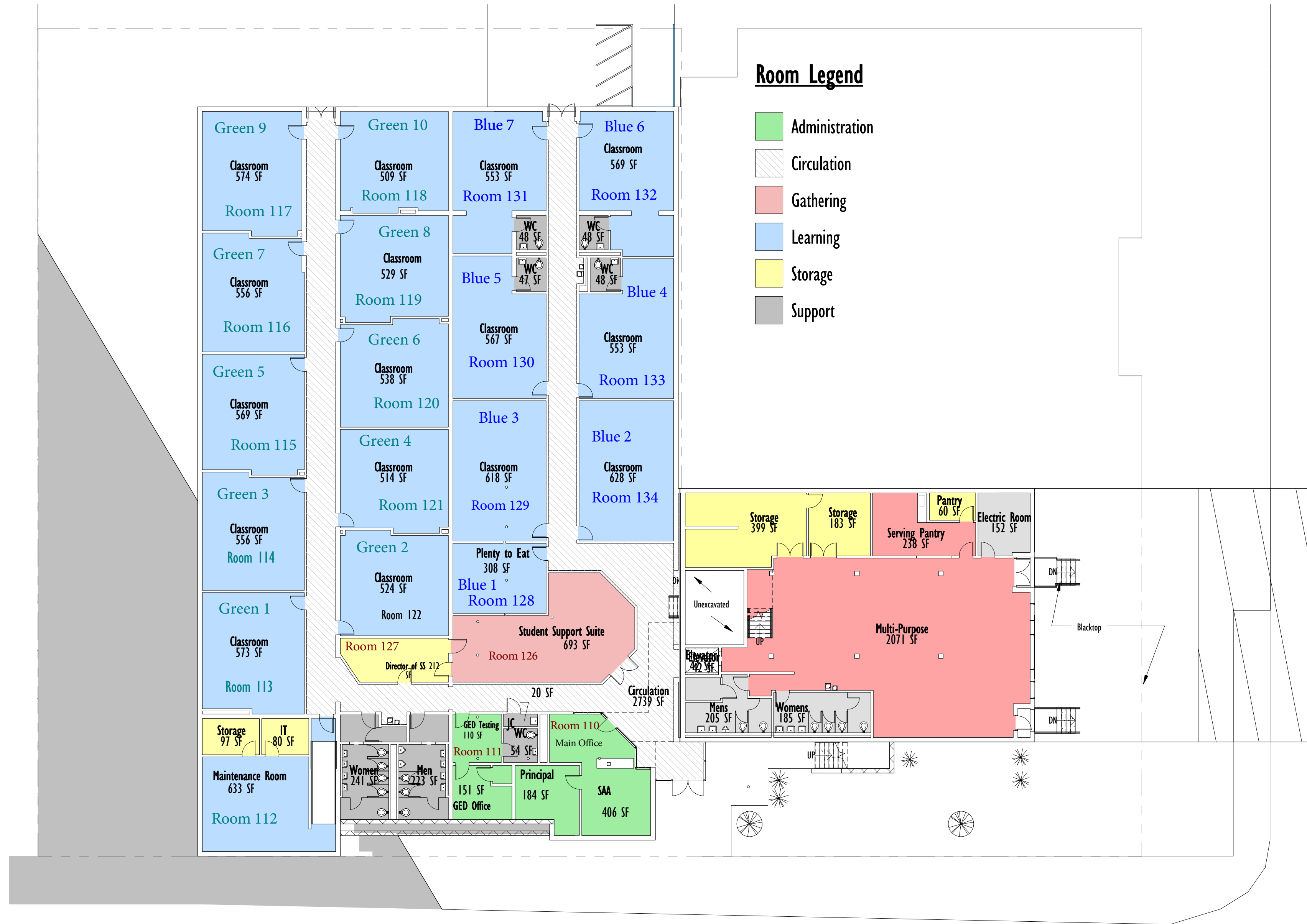
① 01 Existing First Floor Area Analysis 1/16" = 1'-0"
